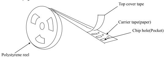
Dimensions of embossed taping for 0805~1812 type
